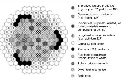
Schematic of FFTF test core, with multiple missions. The hexagonally shaped ducts contain fuel rods, control rods, isotope production experiments, fuel tests, and so on. Production of some isotopes requires slower neutrons, which is achieved by placing appropriate materials around the irradiation target. Some of the test locations are designed to have direct-contact instrumentation during the reactor operation, for example, for rapid retrieval of short-lived isotopes.
