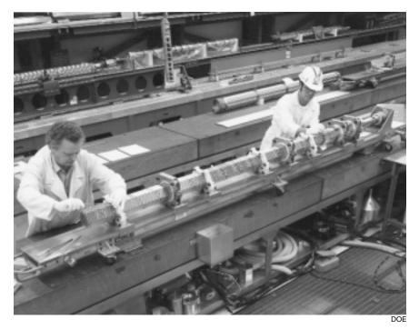
FFTF technicians in 1986, working on a fuel assembly. Each fuel pin is less than a quarter-inch diameter and about 8 feet long. The fuel pins are gathered into 217-pin assemblies, like the one shown here, which are housed in hexagonally shaped ducts in the reactor core.
